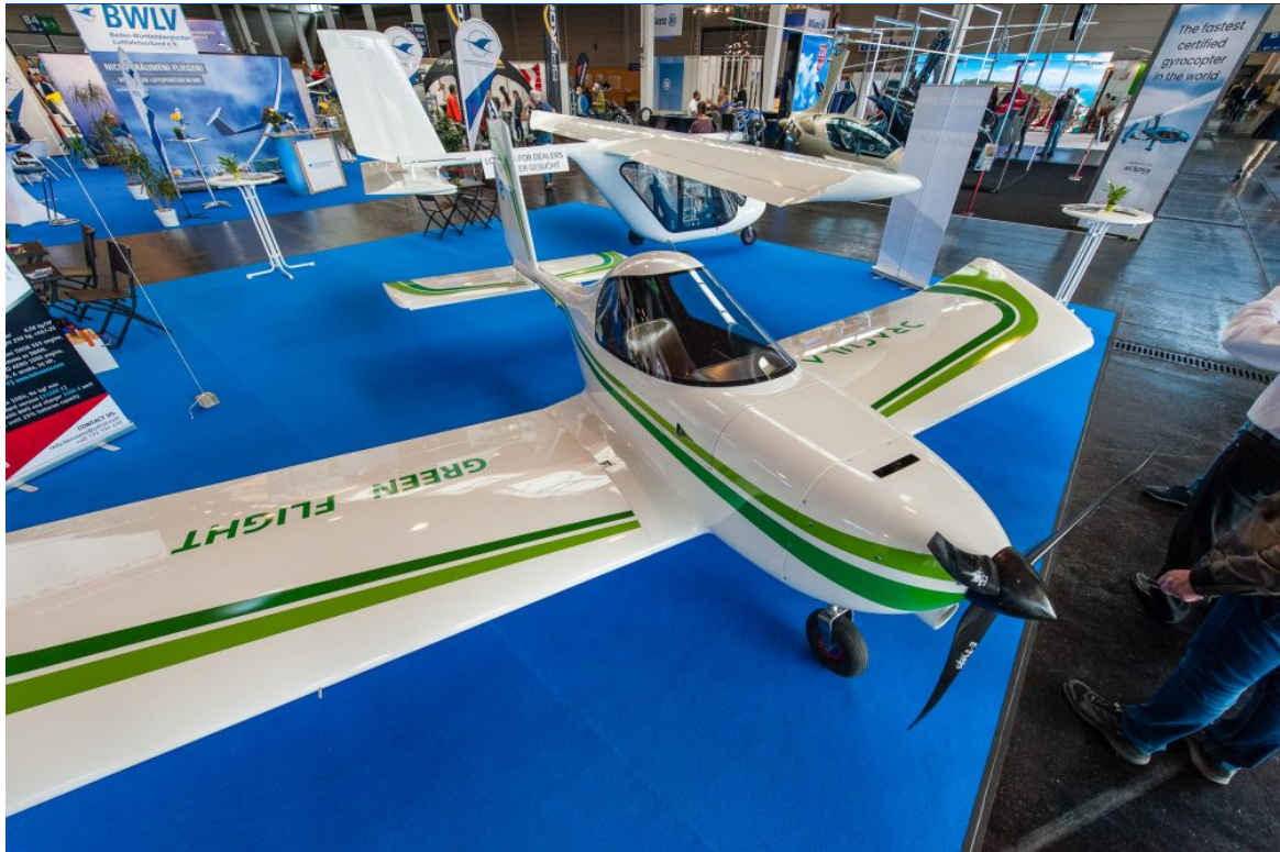
The Swan S500 known as the 'Dracula' powered by either a 30hp petrol engine or electric motor. The giving (or taking of) blood isn't essential...
