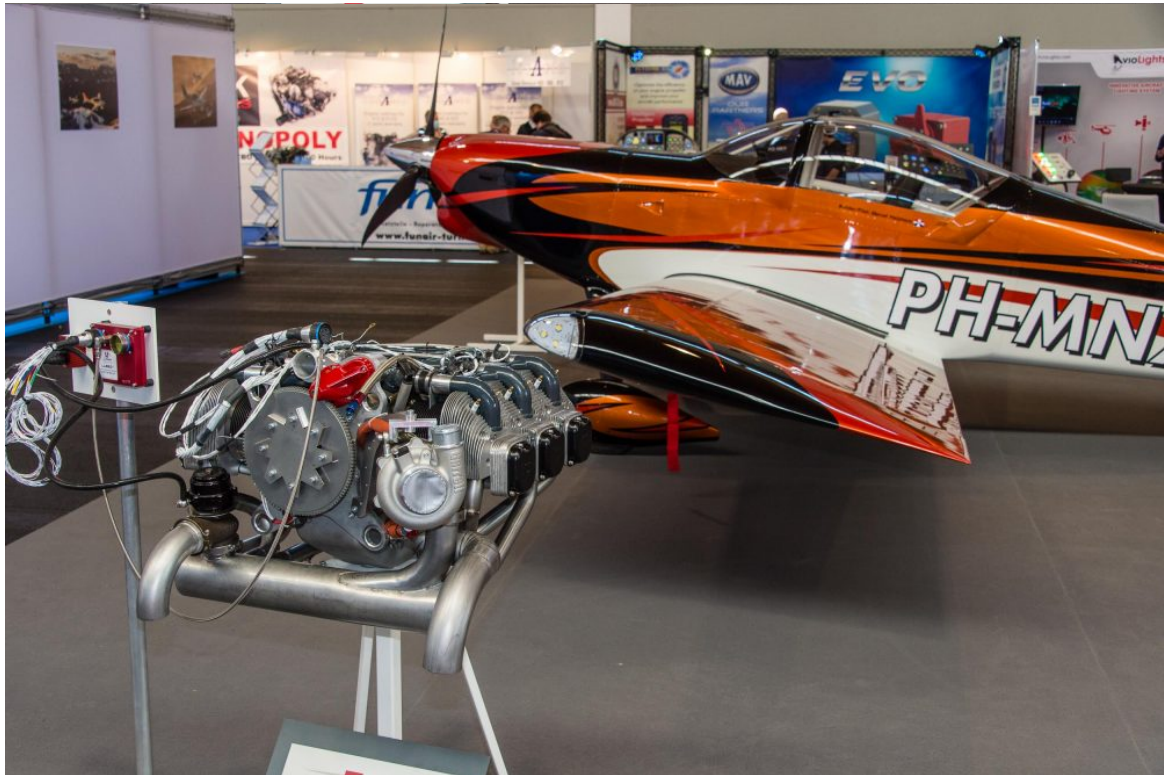
ULPower's latest engine is the UL520T. It's turbocharged but just to 'normalise' it for higher altitudes. Max power is 220hp up to 15,000ft.
