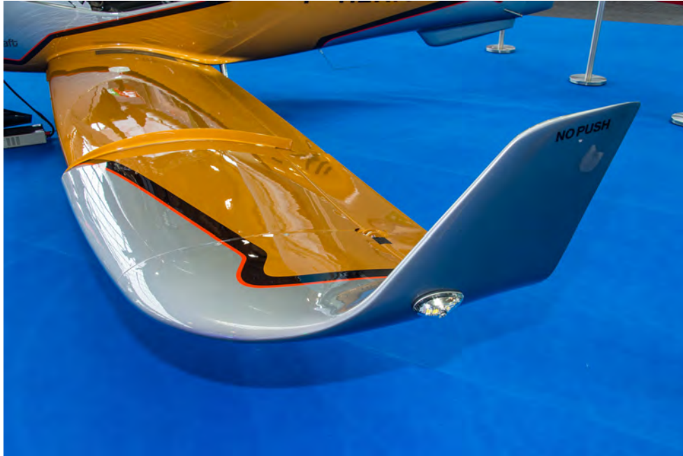
Bigger wingtips and a longer wing are fitted to the 915iS Elixir to maintain its spin-resistance. Photos: Ed Hicks
