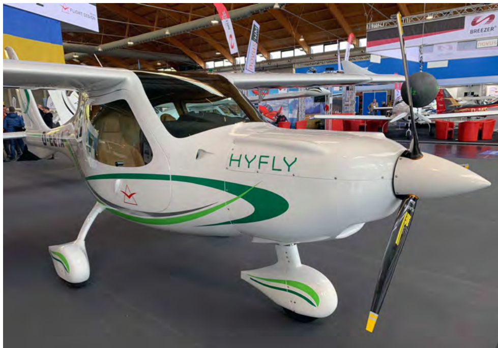
The hydrogen fuel cell powered Flight Design F2. Top photo shows the under fuselage air intake
