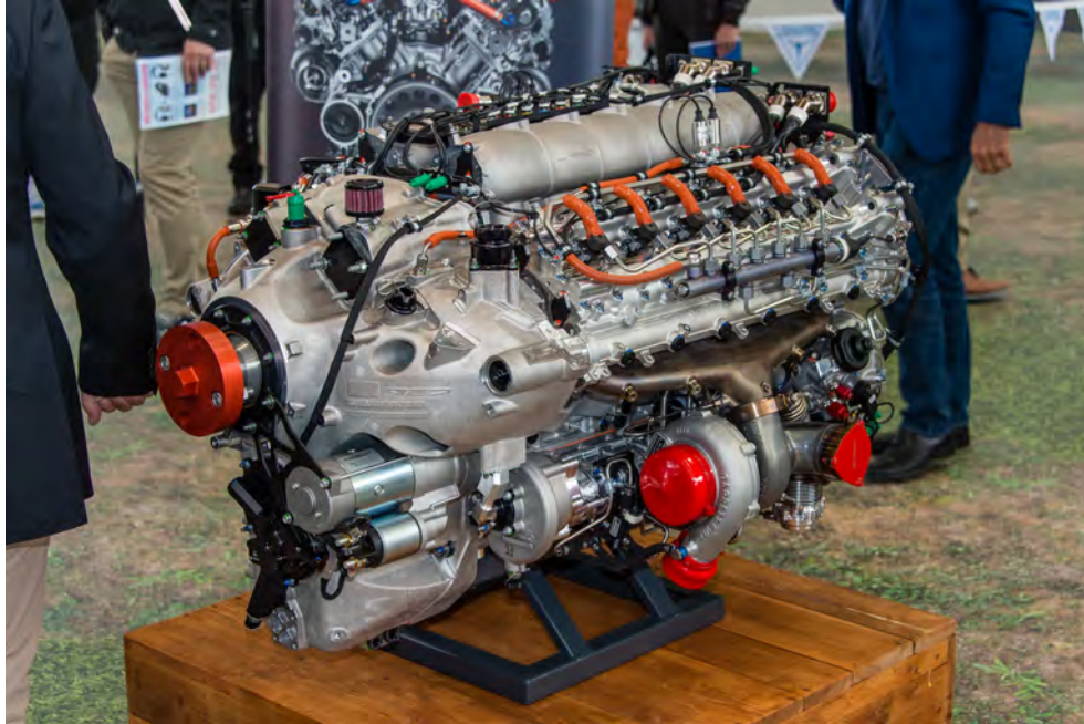
The JU-52 NG will have modern engines – the 550hp RED A03-005 V12 diesel
