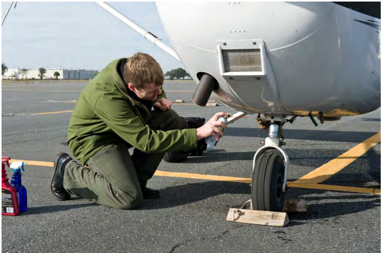
Undercarriage legs must be kept clean and well-lubricated to function normally
