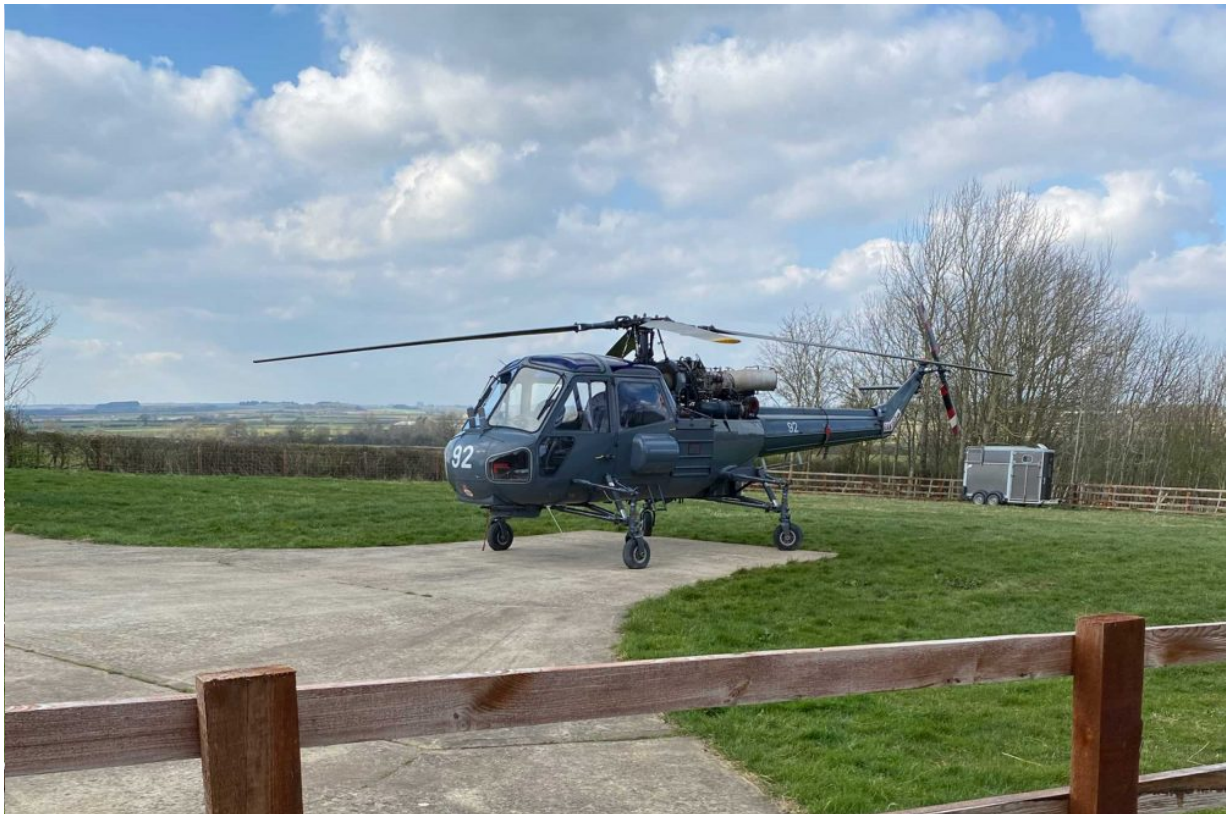
Royal Navy preferred wheels undercarriage for its Wasp, so it could be easily pushed around on board a ship
