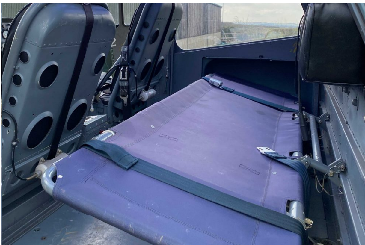
Both aircraft have stretchers for back seats, with the rear doors extended out to accommodate them
