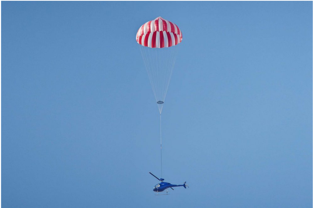
Zefhir helicopter being tested with the whole aircraft ballistic parachute. Curti has moved the 'chute from on top of the main rotor to the fuselage
