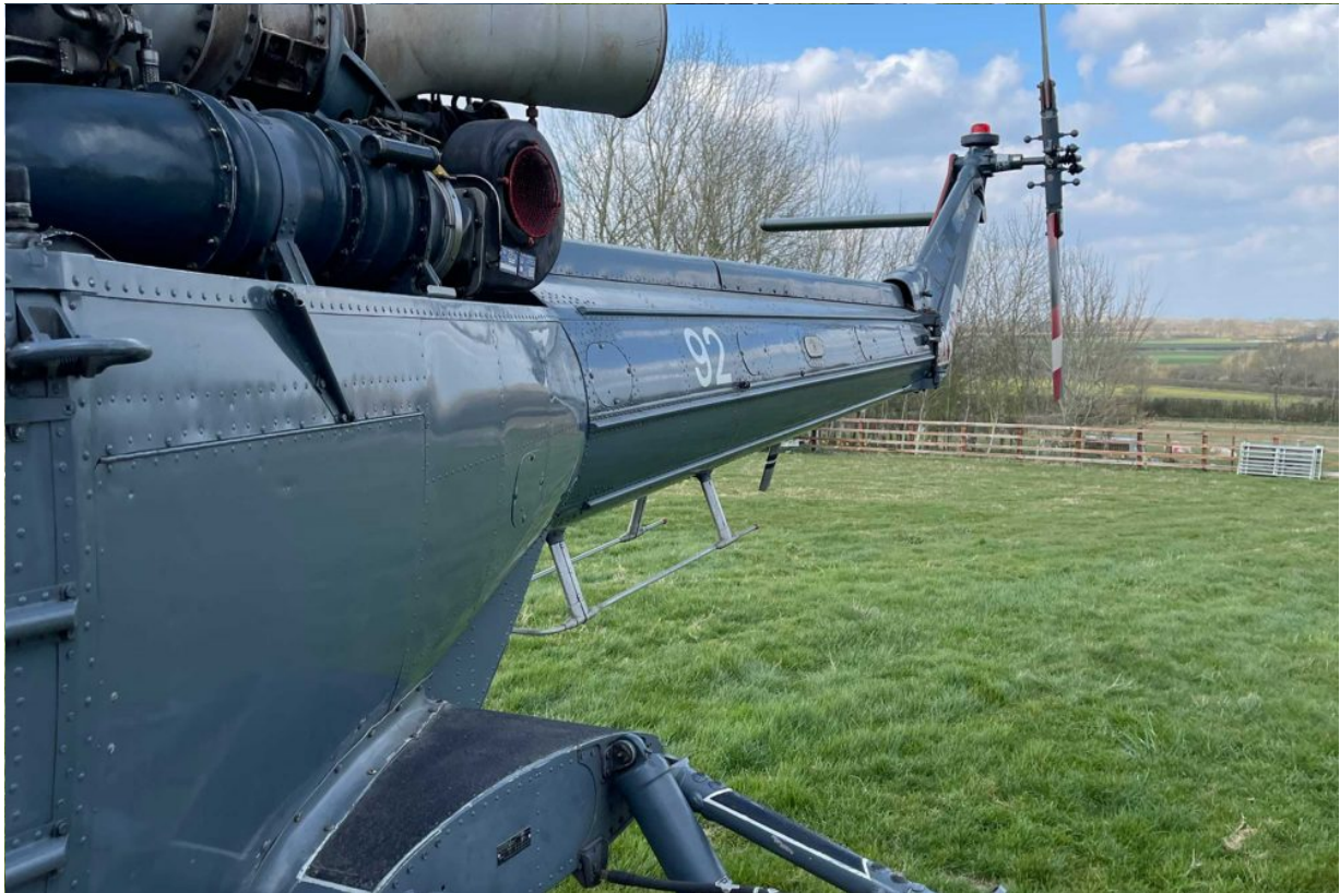
The Wasp has a distinctive tailplane on the starboard side of the tail rotor
