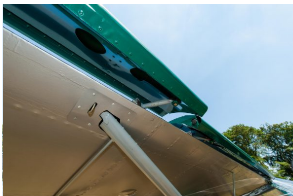
Super-smooth, full-span leading-edge slats
