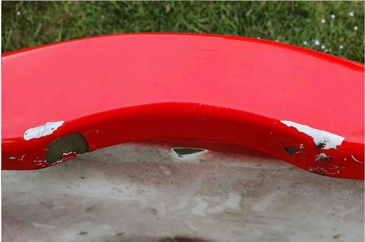
Vibration damage to cowling...
