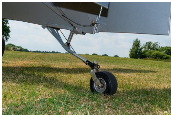
Even the tailwheel has 350psi gas-strut suspension
