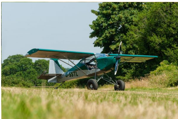
The gas-strut gear and big tyres make simple work of rough ground
